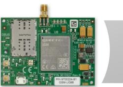
The CLM302 is a penta-band, 3G, dual-SIM cellular add-on that allows the **FORCE** and **FORCE** Lite alarm systems<sup>1</sup> to communicate over a cellular network. The add-on is mounted on the control panel's circuit board and is supplied with an antenna.
