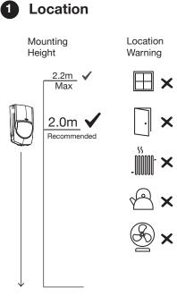
Note: For maximum detection range, especially at high temperatures, mount at 2.0m.
