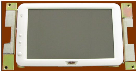
Figure 5. The keypad inserted into the wall box
