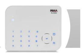
The KLA500 is a hardwired keypad arming station designed for the **FORCE** and **FORCE** Lite intruder alarm systems. It is used for arming and disarming the alarm system and activating devices, and connects to the control panel's bus.
