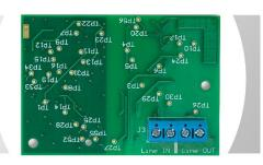
The VPT/VPR500 is a PSTN module of the **VISION** wireless alarm system, which allows it to connect to PSTN network. The VPT500 has Line IN/Line OUT terminal block connector, and the VPR model has RJ11 sockets. A green LED supplies off-hook indication.
