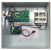
ZEP608 is an 8-zone expansion card (ZEX508) with a 2.0A power supply and a charging card PSC604, mounted in a metal enclosure with a tamper switch.
